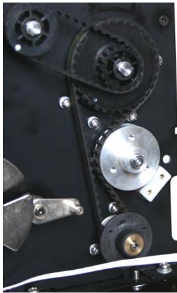
The Toothed Belt path with the Optical Encoder Disk Assembly removed to ease viewing
